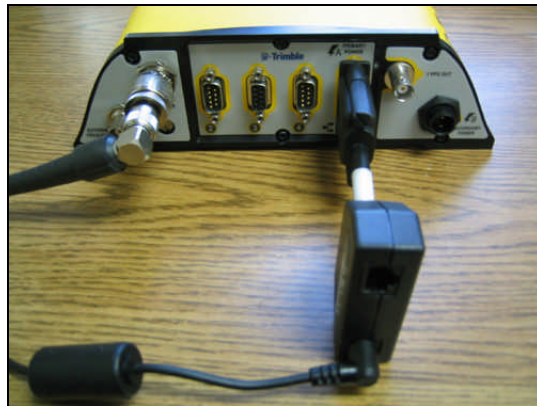
Figure 6. Back Panel Antenna and Power Connection
