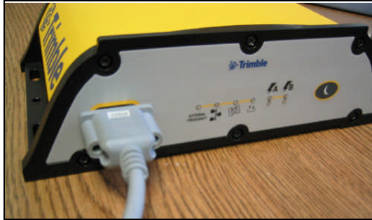
Figure 5. Front Panel Service Port RS-232 Connection
